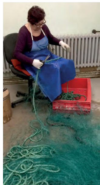
Brugte garn fraskæres. / Old lines are cut off for remounting.
